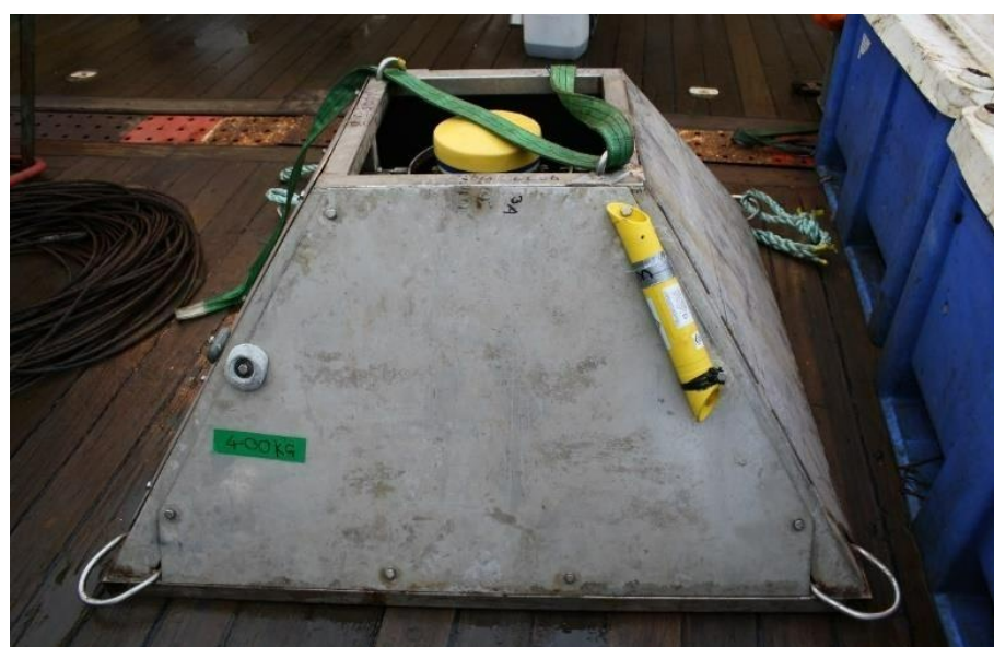
Example ADCP seabed frame for metocean surveys
